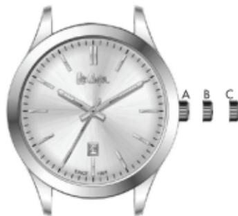
\*In case your watch has a threaded watch crown, pull it up by loosening it before the process. After you completed the process, press strongly and place it back by rotating it.
