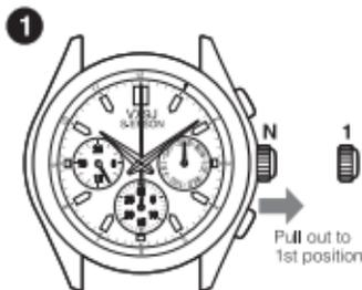
Pull the crown out to the 1st click position when the second hand is at the 12 o'clock position.
