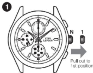
Pull the crown out to the 1st click position when the second hand is at the 12 o'clock position.
